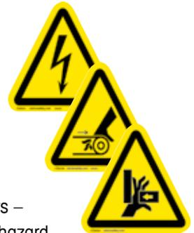
ISO 3864 is the latest standard dealing with this topic, and its method to define the level of risk through a signal word and a background color is accepted for global practice. Those two elements – hazard icon + signal word – in combination, can usually address the notification needs for most hazard zones.
